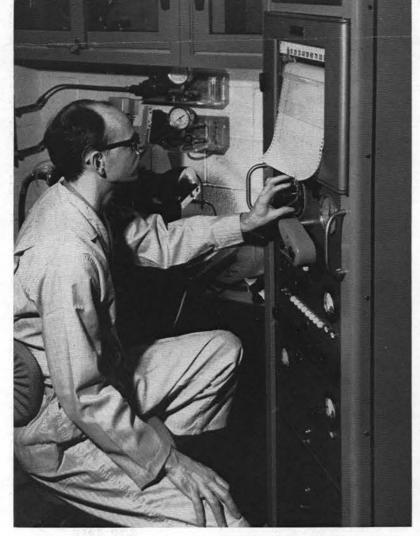
X-RAY SPECTROPHOTOMETER, operated here by Lee Klaus, can identify most any substance from only a few milligrams.
